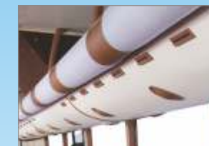
Modular hatrack with integrated AC duct
