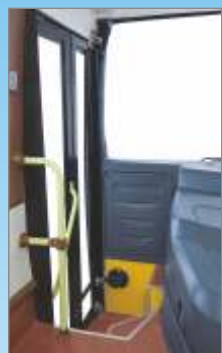
Pneumatic passenger door with sensitivity (AIS052) for safe entry & exit
